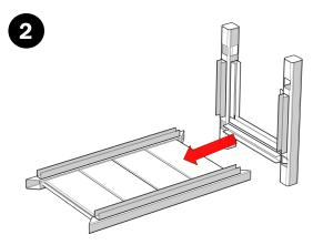
Continue by placing this group onto the Floor Section.
