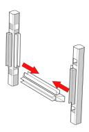
Place Posts onto the short side Rails which contain (2) Side Channels.
