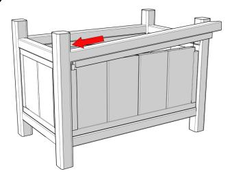
Now, place the Rails with (1) Channel onto the Panels, and into the routed Post holes.
