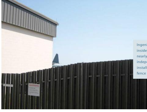
Ingeniously simple design places the rails inside the panels, so your fence can rack to nearly any landscape contour. Each panel can be independently staggered for a perfect "stairstep" installation that is unattainable with other sectional fence products.
