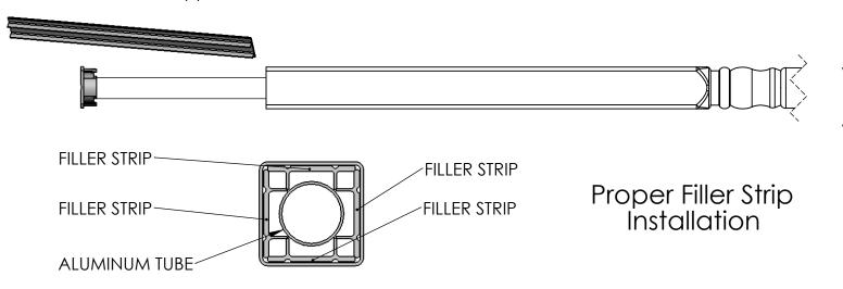
6) Slide the Decorative Column over the Filler Strips and down onto the Mounting Plate until they sit flush as shown.
